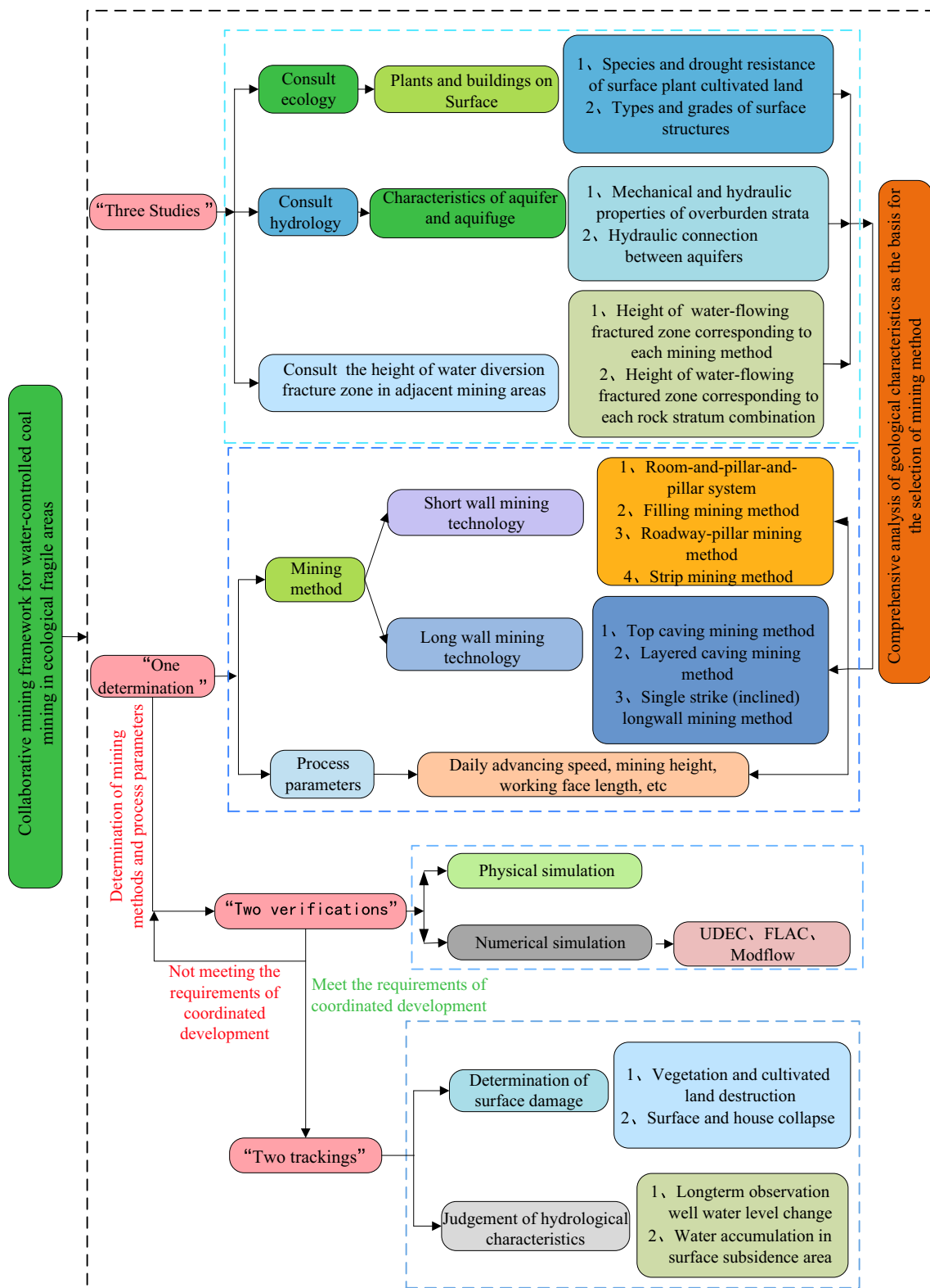
Fig. 9 Collaborative mining framework of water-controlled coal mining in ecologically fragile area
